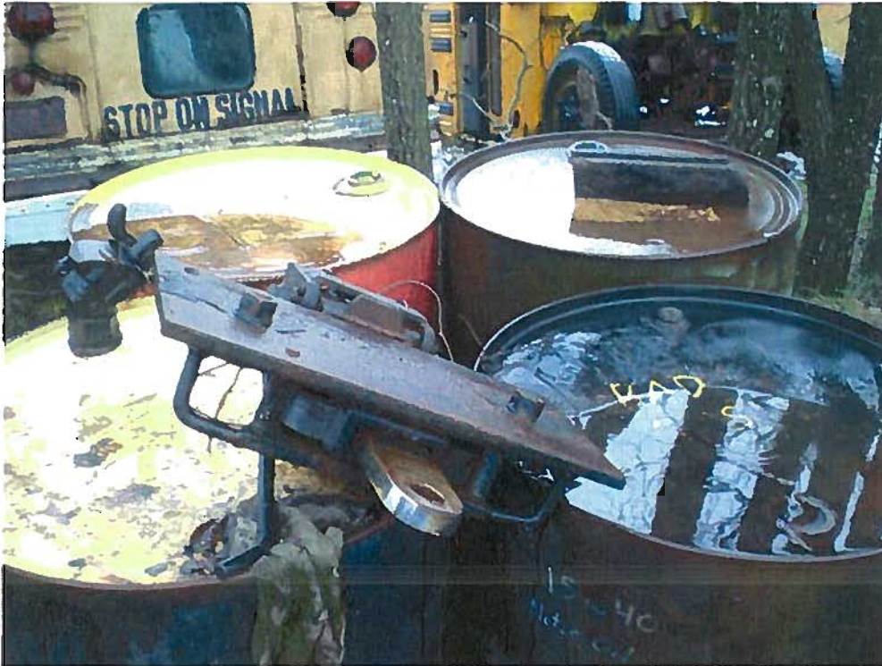
Date: 11-29-2011 Time: 2:59pm Direction: W (down) Photo by: P. Fatka Exposure #: 025 Comments: View of the tops of the barrels showing they are holding water and rusting.
